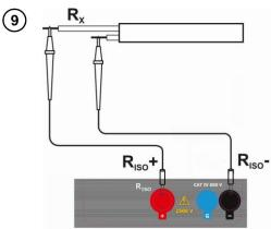
Connect test leads according to the drawing.
