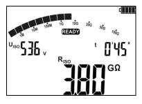
After the measurement is completed or stopped, read the result. The results of all completed measurements will be displayed (even when the measurement was interrupted/stopped e.g. after 60 seconds). When the meter switched into standby mode, the measurement result may be recalled by pressing ENTER.
