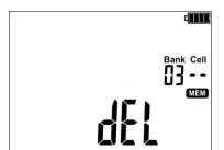
... and the cell number will change into "--", then symbol del will be displayed to indicate the readiness for deleting.
