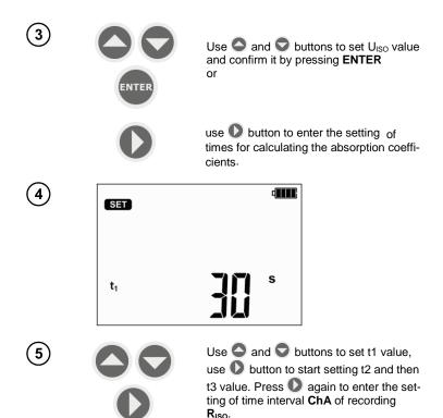
Defining ChA interval will enable the user, using Sonel Reader software, to plot the resistance chart and current chart using the data obtained from the performed measurement (see example below).
