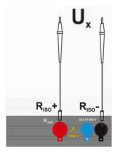
Connect the meter to a voltage source.
